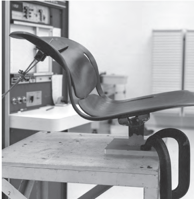
2. Equa Chair on test rig
